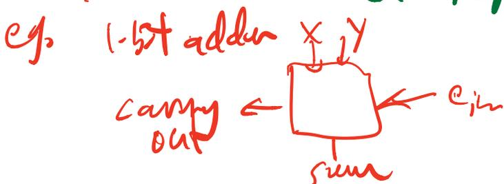
$$\begin{aligned} \text{sum} &= X \oplus Y \oplus c_{in} \\ c_{out} &= \text{maj}(X, Y, c_{in}) \end{aligned}$$
